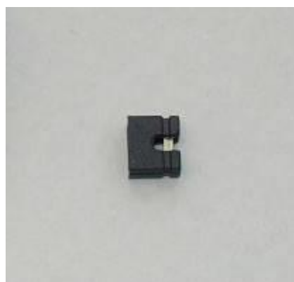
Picture 2-14: Jumper for disabling the sampling clock oscillator
