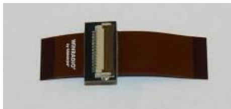
Picture 2-7: Digital synchronization cable for the WR-G35DDCi receiver, unused in the ETC configuration (see text)
