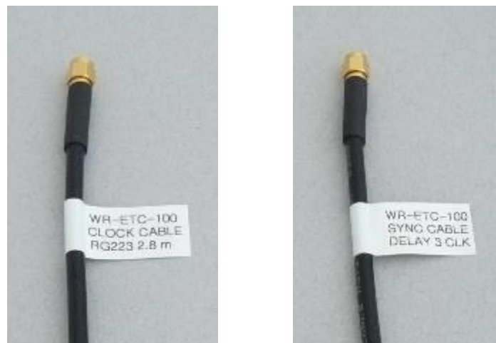
Picture 2-20: Note the labels of the CLOCK SMA coaxial cable (on the left) and of the SYNC SMA coaxial cable (on the right) supplied with the ETC kit. The DELAY specification is stated on the SYNC cable shown on the right – this particular cable shown in the picture has the delay specified as "DELAY 3 CLK". That means the cable delays the signal by 3 sampling clock periods. The value of the delay has to be specified in the software, so that the software can compensate for the delay.
