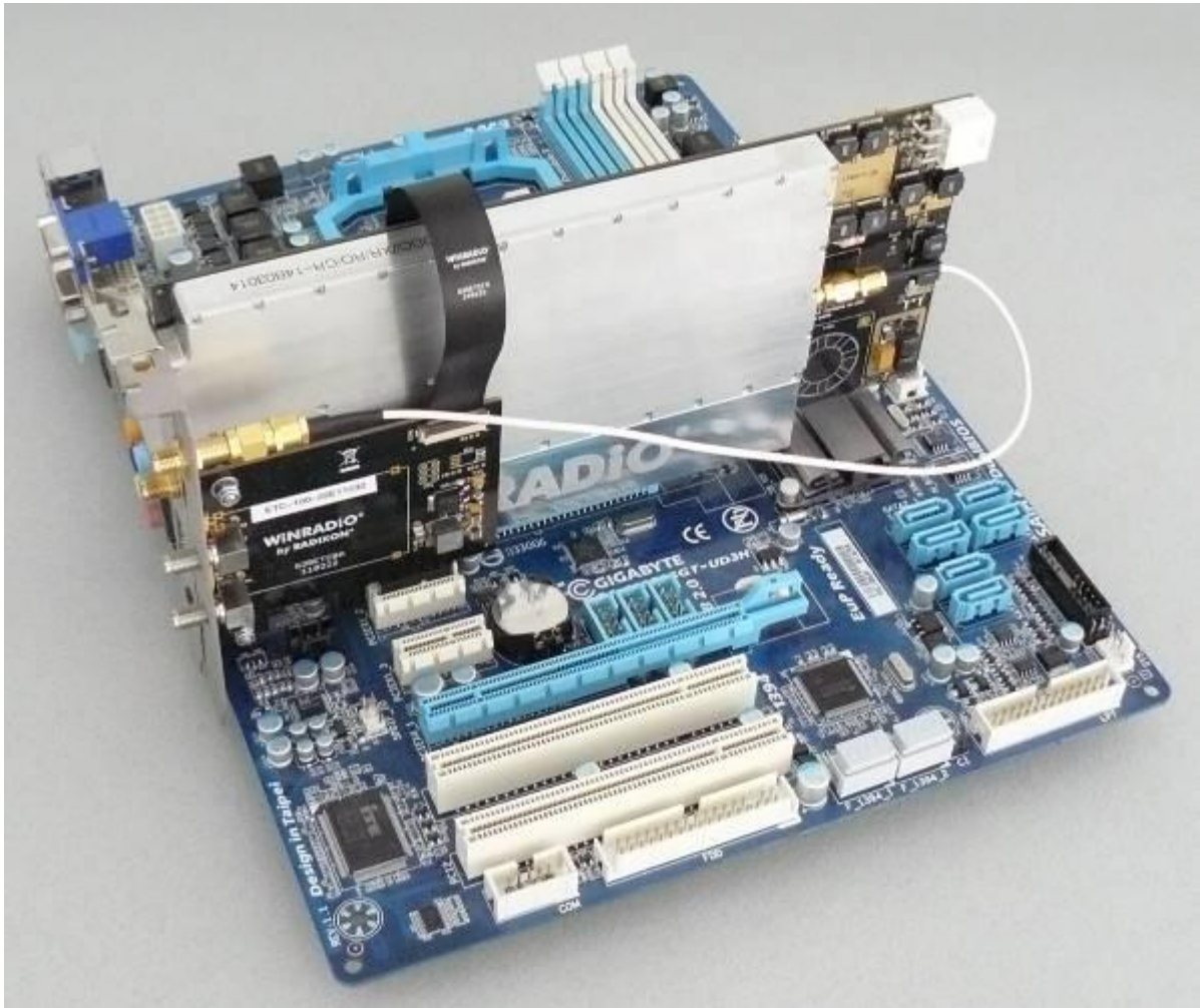
Picture 3-8: The completed installation of the ETC board into the PC next to the receiver.
