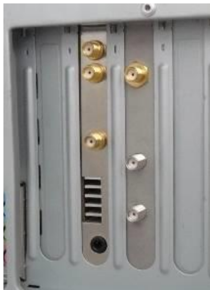
Picture 3-9: The completed installation of the receiver (shown on the left) and the ETC board (shown on the right) fitted into the PC as seen from the rear of the PC.
