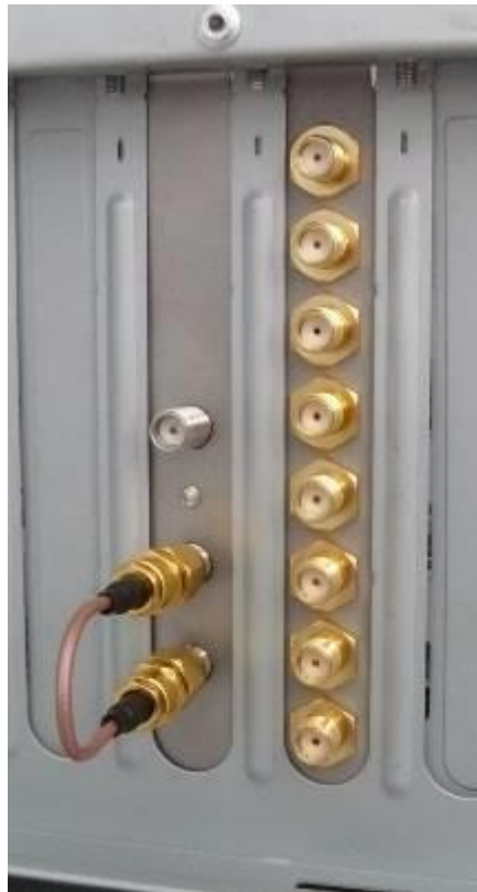
Picture 3-13: Installing the frequency reference SMA interconnect cable for internal frequency operation
