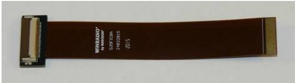
Picture 2-8: Digital synchronization cable for the Coherent clock generator board, unused in the ETC configuration (see text)
