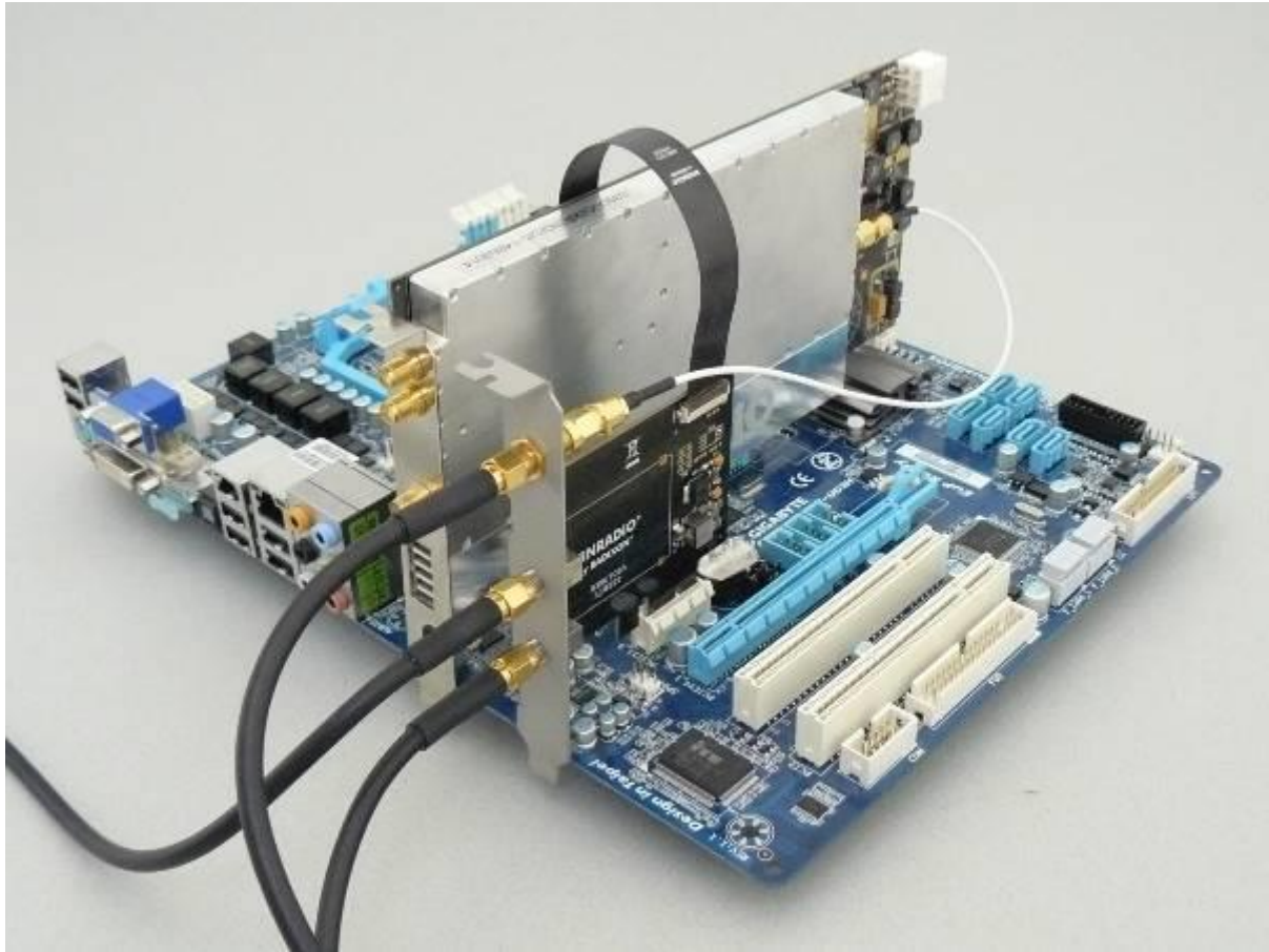
Picture 1-2: An example of a one WR-G35DDCi receiver, forming part of a multichannel coherent system in ETC configuration with the ETC kit, installed into a PC (PC chassis and other PC connections omitted for clarity). The WR-CC1PPS-100 kit is also required for coherent operation, but is not shown in this picture.
