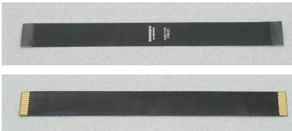
Picture 2-17: The Digital synchronization flat cable for the ETC board front view (top) and back view (bottom)
