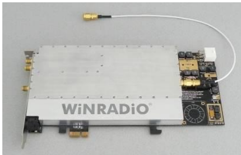
Picture 3-3: Sampling clock patch cable installed onto a receiver
