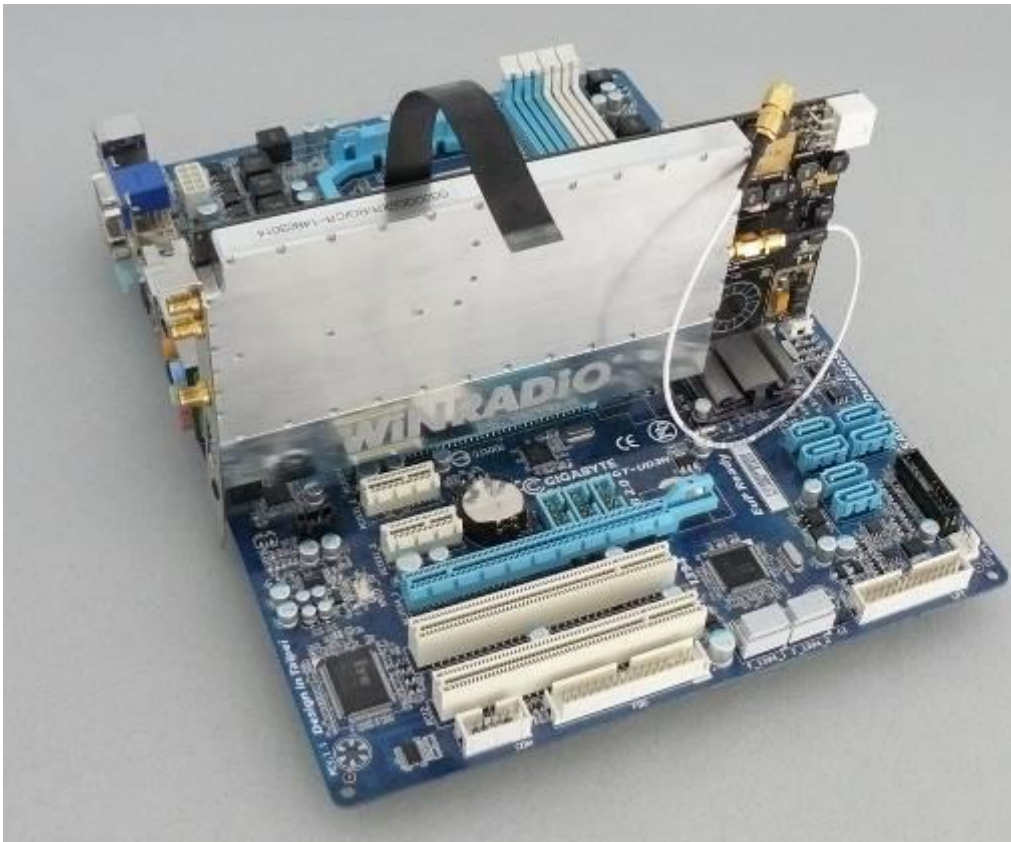
Picture 3-6: A receiver is installed into the PC, showing other ends of the flat synchronization cable and SMA coaxial clock cables unconnected.
