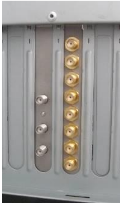
Picture 3-12: The completed installation of the Coherent Clock Generator board (on the left) into the PC together with the PCIe bracket multi-SMA adapter (on the right) installed next to the Clock Board as viewed from the rear side of a PC.
